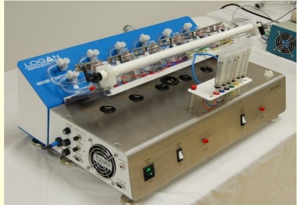
For media replacement, the cell support plate tilts to purge any bubbles
