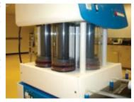
the volume accuracy is within 2% for media transfer under 500ml and better than 1% for the transfer media above 500ml.
